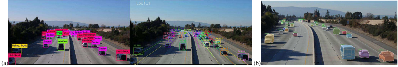
Figure 2: Highlights of Track 1 methods. (a) Team 48: left: detected vehicles with car types, right: vehicle trajectories with estimated speed in MPH. (b) Team 78: Vehicle detection using Mask R-CNN.
