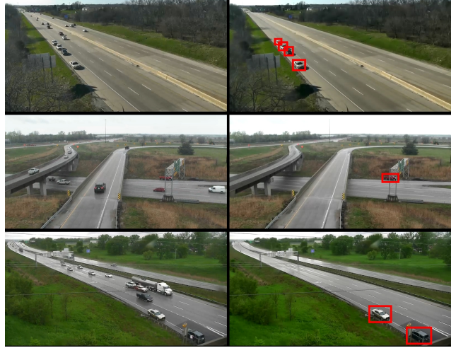
Figure 5. Examples of detected anomalies on the Iowa DOT Traffic Dataset. Original video frames are shown on the left, and processed videos frames with detected anomalies from [39] are shown on the right.
