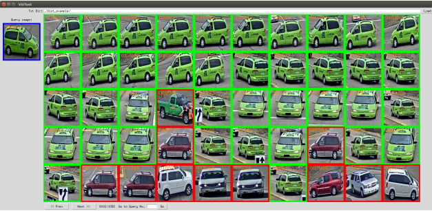
Figure 4. User interface of the Python visualization tool for qualitative evaluation on CityFlow-reID. Green and red rectangles represent true and false matches, respectively. This visualization is only available from the challenge organization, as the plotting requires ground truth.
