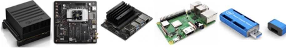
Figure 4: Hardware: NVIDIA Jetson Xavier, NVIDIA Jetson TX2, NVIDIA Jetson Nano, Raspberry, Intel NCS 2
