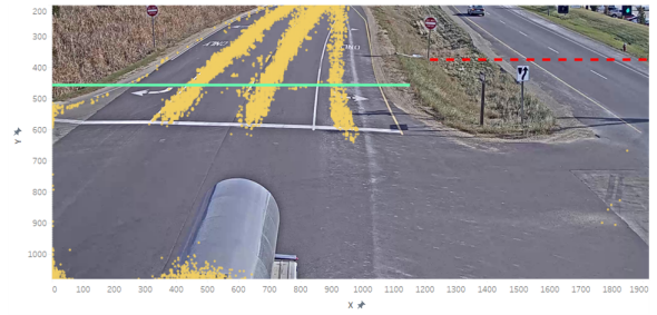
Fig. 2. Virtual representative line generation example: Yellow points indicate no vehicle displacement points, Green line represents the VRL for vehicles of the query dataset, Red-dashed line represents the VRL for vehicles of the gallery dataset
